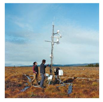
INSTRUMENT TOWER measures carbon dioxide and methane transfer between the air and soil year-round, indicating whether the ecosystem experiences a net gain or loss of gases annually.
